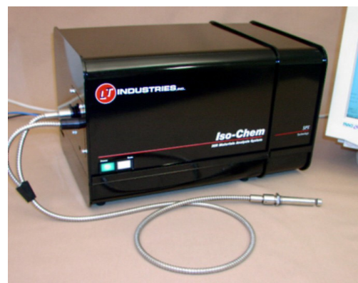
The Iso-Chem system with a fiber optic bundle and a transreflectance probe.
